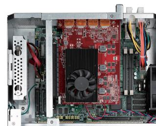
DPX-S1000 internal view with graphic card fitted
