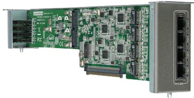
The ITAM-NC02-C copper GbE module is compatible with ITA-22 series systems and supports flexible configuration.
